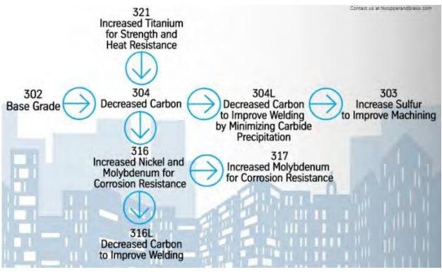
The 300 series stainless steels are classified as austenitic and are hardenable only by cold working methods. These grades of stainless have approximately 18% to 30% chromium and 6% to 20% nickel as their major alloying additions. Austenitic stainless steels are chromium-nickel alloys, which are hardened by cold working. Nickel is the main element varied within the alloys of this class while carbon is at low levels.
