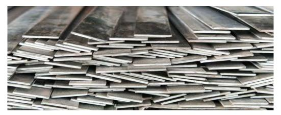
The SS Flat bars are supplied to customers in various thickness from 10.5 mm to 21 mm. The SS Flat bars are made by re-heating the billets and rolling into required size.
